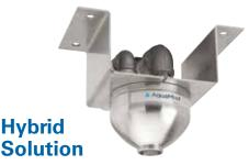
The system operates at less than 9.4 bar (136.0 psi) to produce the smallest droplet sizes of any water mist system, proving that high pressure isn't always needed! The AquaMist SONIC hybrid (water-nitrogen) technology also has sidewall atomisers available for highly obstructed turbine enclosures. The system is safe for people and the environment, and is cost effective to recharge.
