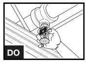
**DO** hand-start sprinklers by gently handling the sprinkler.
