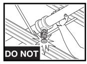
**DO NOT** slide pipe through structure with sprinklers in place.
