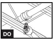
**DO** install sprinklers in sprinkler fittings after sprinkler pipe is in place.
